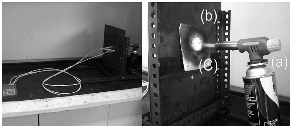
Figure 1. Fire test setup for the heat insulation test of the intumescent formulation: (a) portable Bunsen burner, (b) stand, and (c) sample of intumescent coating.
